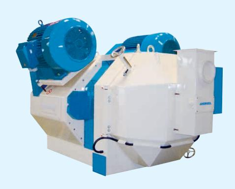
The authentic and sturdy Paladin design is constructed with a balanced twin drive system, where the transmission consists of a combination of V-belts and a toothed belt. The design of the main shaft and rotor allows maximum torque to be applied in the pelleting section. These features make the Paladin pellet mill range universally adaptable machines, en-
